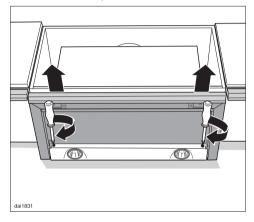
■ The deflector can be adjusted up to 1 <sup>3</sup>/<sub>8</sub>" (35 mm) towards the front with the two adjusting screws left and right in the deflector. Adjust the deflector until it is flush with the front of the adjacent cabinetry.
